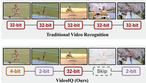
Figure 1: A conceptual overview of our approach. Instead of processing all the video frames with the same 32-bit precision, **VideoIQ** learns to dynamically select optimal quantization precision conditioned on input clips for efficient video recognition. It is computationally very efficient to process more informative frames with high precision and less informative ones with lower precision, without sacrificing accuracy. Best viewed in color.
